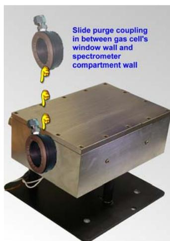
The Purge Couplings (14) should then be inserted in between the gas cell body and the spectrometer sampling compartment. The gaskets should be compressed slightly to ensure intimate contact and an effective seal. The better this seal is made, the better the purging and in turn the better results you will achieve in collecting spectra. Each purge coupling has two 1/4" Swagelok nozzles for affixing the purge gas lines.
