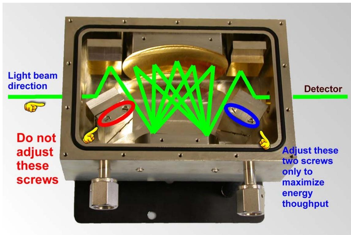
3. Before placing the Cover Plate (1) back into the gas cell, make sure that the o-ring that provide sealing between the cell body and cover plate is clean and without any type of debris.
