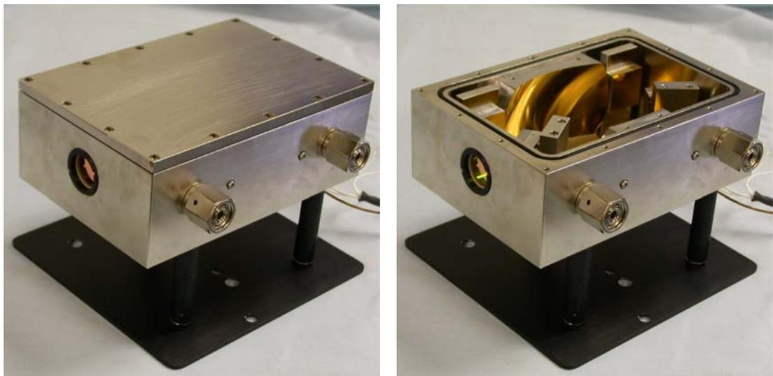
2. Starting with the exit "Transfer Mirror" and using a small blade screwdriver, make small adjustments on the two controls of the mirror position to maximize the energy; repeat this process in cycling between the two controls until a final maximum is obtained.
